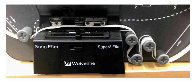
Note the dotted lines. Wrap film loosely and carefully to follow the pathway as illustrated above. The film should be comfortably loose at this point.
