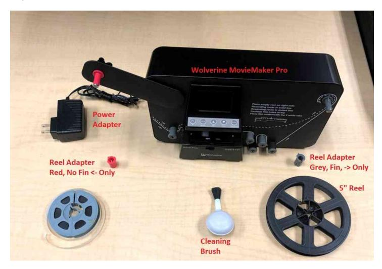
Relevant parts include the MovieMaker Pro itself, the 5" Reel (aka Take Up Reel), the Power Adapter, and the reel adapter. There is also a cleaning brush included in the kit.
