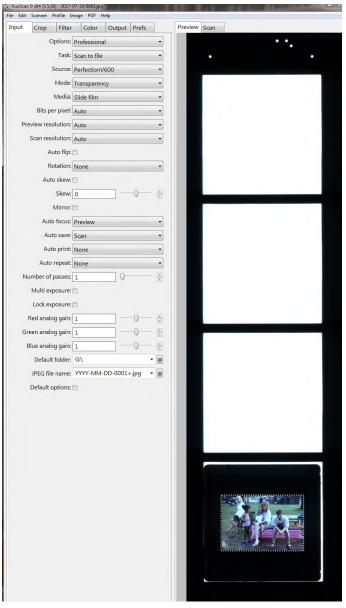
You can MOUSE over the dotted line until to see a double sided arrow, HOLD DOWN the LEFT BUTTON and drag the dotted line to the outside line of the picture. Select carefully as it can affect the scan quality if you select outside the actual transparent media.
