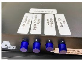
The process is the SAME as VHS to Electronic File, except you use the correct player for your 8MM tape. You also must select the right input using the 4port switch box AND the 8mm will only display on the RIGHT monitor.
