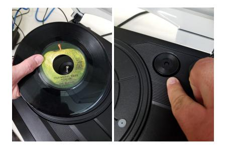
**Step Five**: When the track is queued up, press the record button in the AUDACITY program, then turn on the POWER of the JENSEN PHONO PLAYER. The turntable should then start spinning, and record activity will be shown on the AUDACITY screen.
