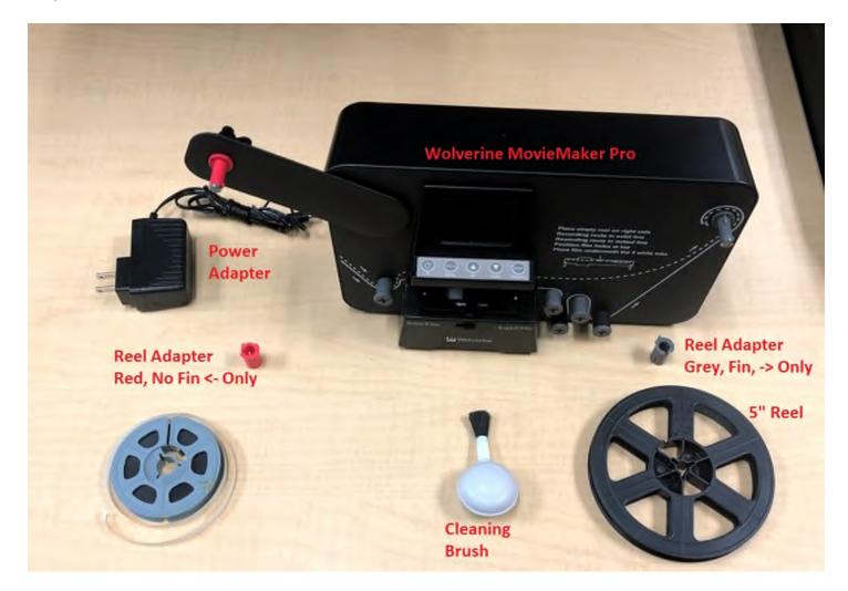
Relevant parts include the MovieMaker Pro itself, the 5" Reel (aka Take Up Reel), the Power Adapter, and the reel adapter. There is also a cleaning brush included in the kit. (This illustration shows a RED ADAPTER, but that was LOST previously and is NOT REQUIRED.
