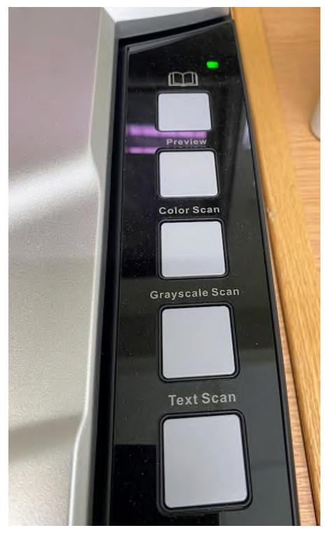
Located on the RIGHT side of the Scanner are 5 "quick" hardware buttons that perform the same functions as listed under Step 5 EXCEPT they're "automatic"
