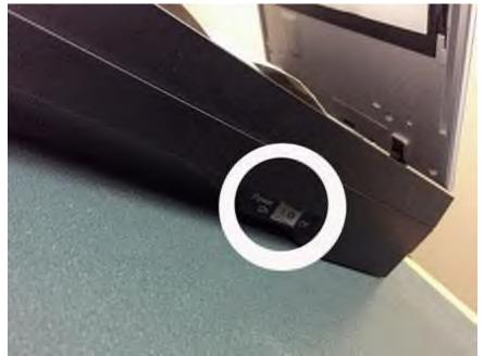
The scanner MUST be powered on BEFORE starting the VueScan x64 software. Failure to turn on the scanner will require you close the software and reload it. This step is necessary for the software to detect the scanner.
