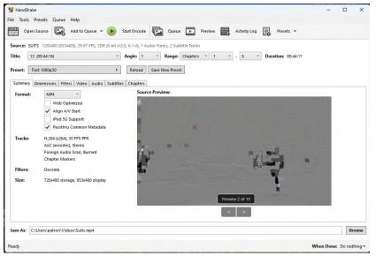
The DEFAULT format is MP4 and we strongly recommend using that. There are no real changes needed to produce a decent MP4 file.
