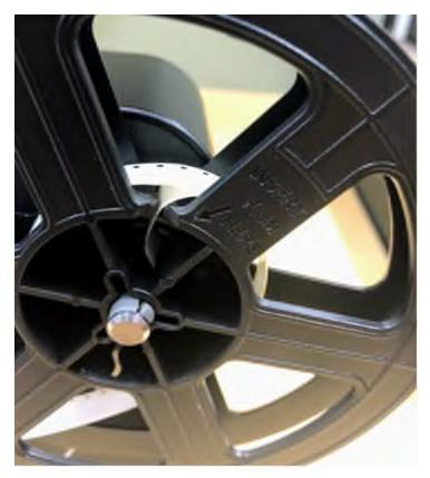
Place end of leader film into the notch marked "INSERT FILM HERE" and then rotate your takeup reel lightly counter clockwise a few times.
