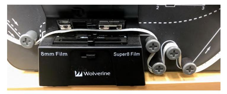
Note the dotted lines. Wrap film loosely and carefully to follow the pathway as illustrated above. The film should be comfortably loose at this point.
