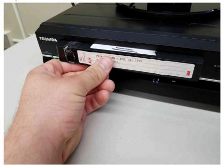
**Step Three**: Press the SELECT so VCR is highlighted. Use Play/Stop buttons to cue up for VHS tape to where you wish to record from and press STOP.
