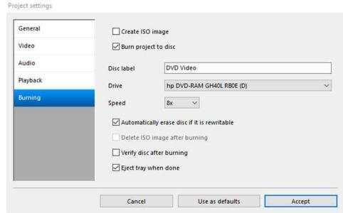
For the last tab, BURNING, you will want to ensure that BURN PROJECT TO DISC is checked, and also ensure that SPEED is set to 8x or higher. It defaults to 4x, which is slow. Do not go higher that 16x.
