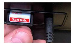
In the back of the Wolverine Movie Maker Pro, plug in the power cable and the SD card as shown below.
