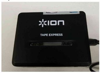
**Step Two:** Plug USB from ION TAPE EXPRESS into the USB HUB. Ensure NO OTHER DEVICES ARE PLUGGED IN.
